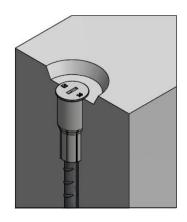
After removing the KU nailing plate, mount the plastic plug inside the socket.
